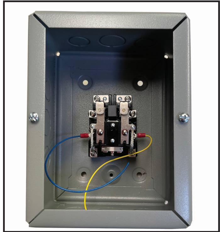
External Contactor Box - This option provides a contactor that can disrupt power for large boilers up to 50 amps 1 1/2 hp
